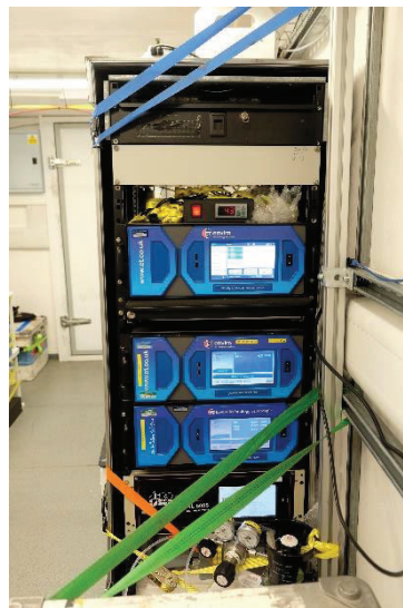
Figure 15. The rack of instruments used during the cruise. The O 3 analyser is missing from this photograph as it was held in a different rack.
